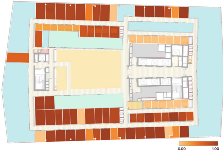
Fig. 8. SVC's prediction probabilities mapped onto an WeWork floor plan. 0.0 indicates when the model is certain the particular office will not be low performing, 1.0 indicates model certainty in low performance. These probabilities can be thought of as model confidence
