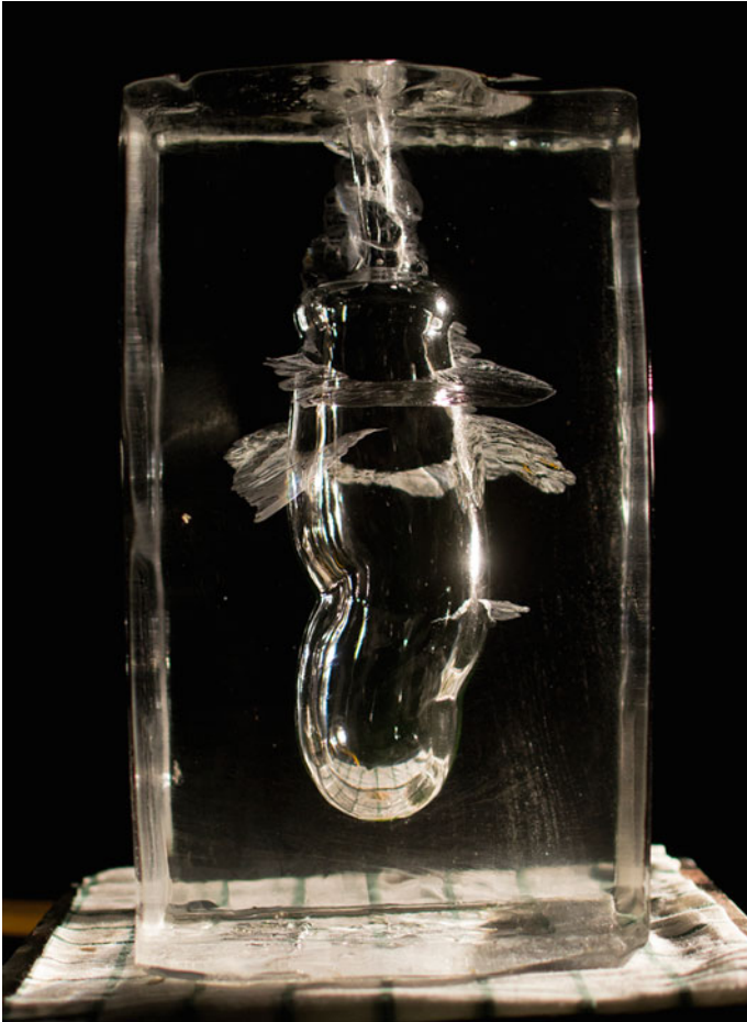
Fig. 9. Melting test #1—the ready formwork (full documentation: goo.gl/FPIMW8 )
