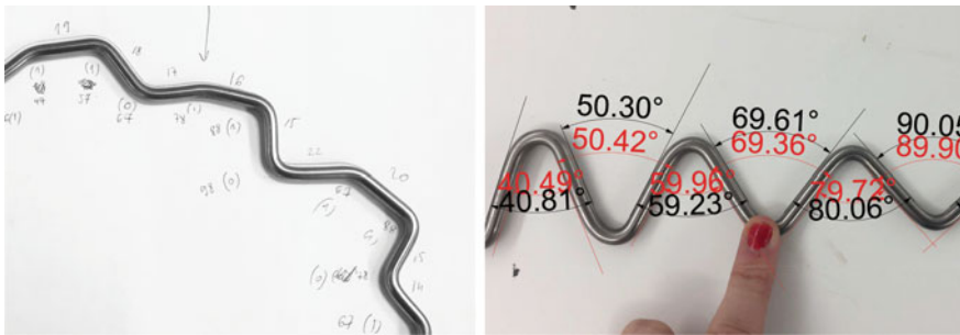
Fig. 10. Left: manual readouts of the bent angles; Right: averaged photo readouts method
