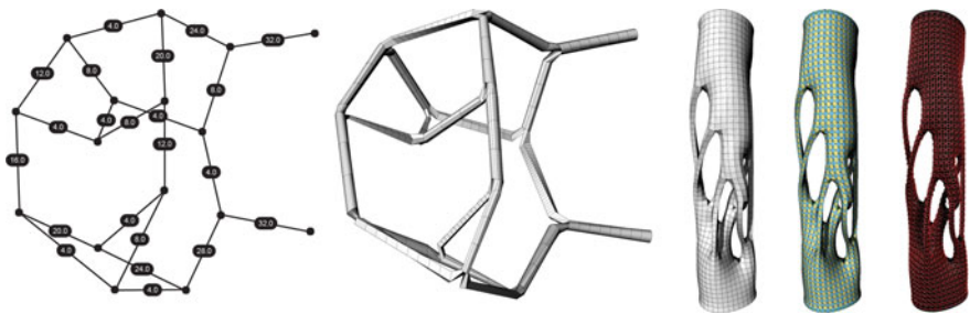
Fig. 10. Example mesh solution ( center ) from a weighted macro scale directed graph topology ( left ) and the eventual result from the braid solver ( right )
