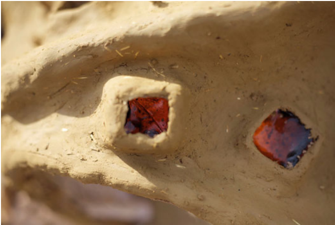
Fig. 9. Natural resin robotic pouring. Earthen Shells’workshop 2017
