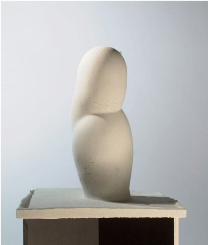
Fig. 4. Melting test #1—a negative cast of the surface developed by projecting a heated water jet onto the surface of ice. Full documentation of the fabrication process: goo.gl/FPIMW8
