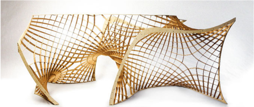
Fig. 9. Model of the design implementation. The structure is built from straight timber strips of beech veneer with exclusively orthogonal nodes. Image and model Denis Hitrec
