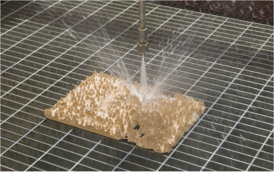
Fig. 1. Erosion-based limestone fabrication process. ©ICD, K. Rinderspacher
