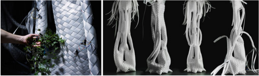
Fig. 2. (left) Braided scaffolds supporting plants and robotic elements in the flora robotica project. (right) Hand braided examples of self-supporting complex braid topologies
