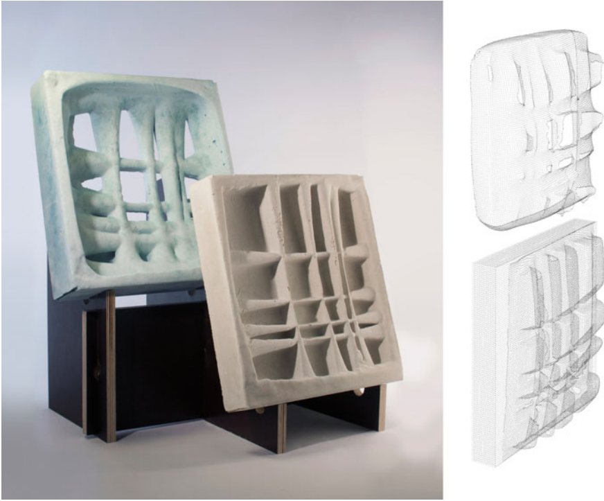
Fig. 6. Melting probes #3—a negative casts of the geometry of the ice surface created through submerging ice in a saline solution of sub-zero temperature. When the geometry of ice was imprinted in concrete it was digitally recovered through 3D scan of the negative concrete casts for further analysis
