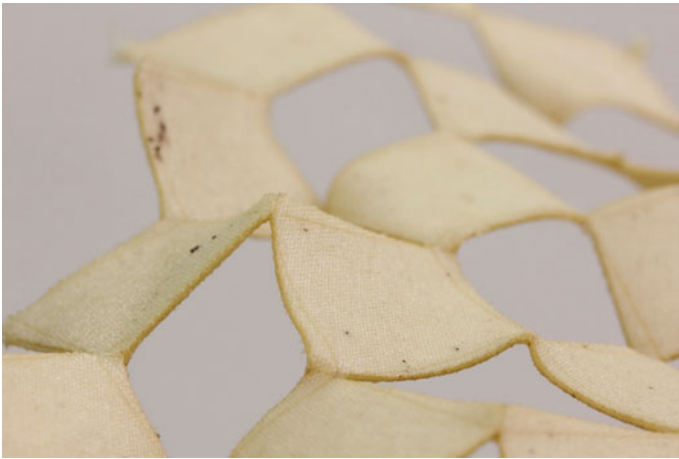
Fig. 16. Matrix made out of resin-impregnated textile based on a quadrangular auxetic structure forming a negative Gaussian curvature (maximal openings 20 mm)
