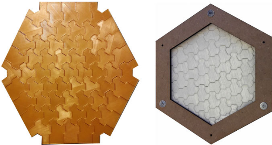
Fig. 11. Type 1 plate (left). Type 2 plate in its test frame (right)
