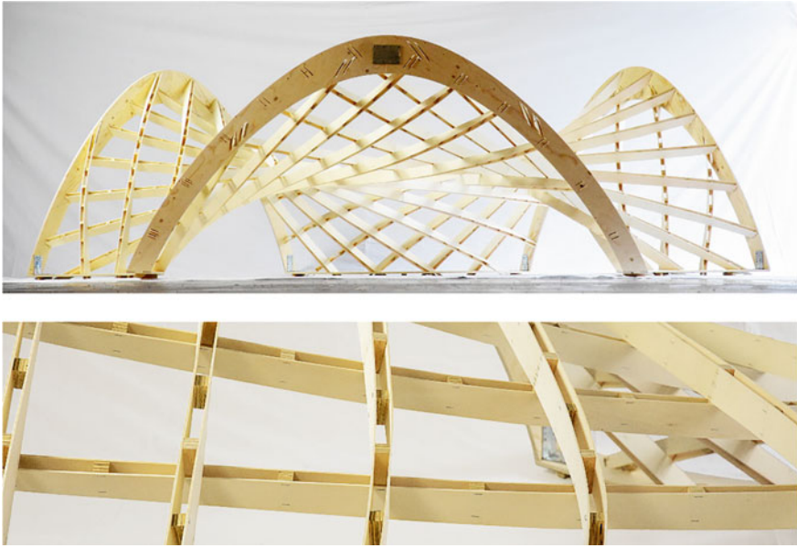
Fig. 10. Timber prototype. The lamellas are doubled and coupled to allow for low bending radii and high stiffness. Image Eike Schling
