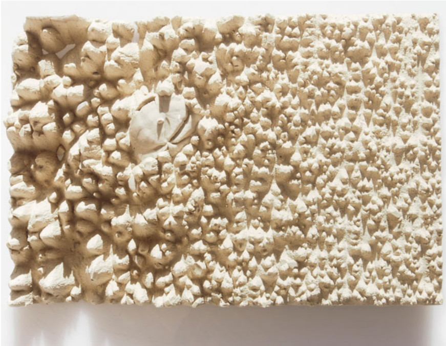
Fig. 5. Limestone sample displaying results from a gradation of water pressure. ©ICD, K. Rinderspacher
