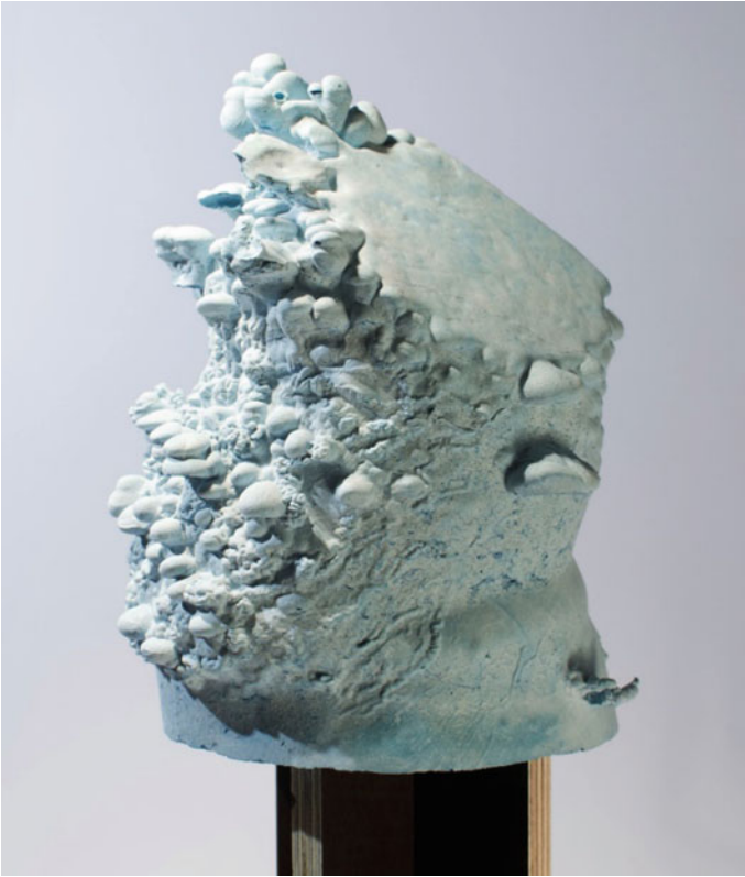
Fig. 5. Melting probe #2—a negative cast of the surface molten by static contact with warm water
