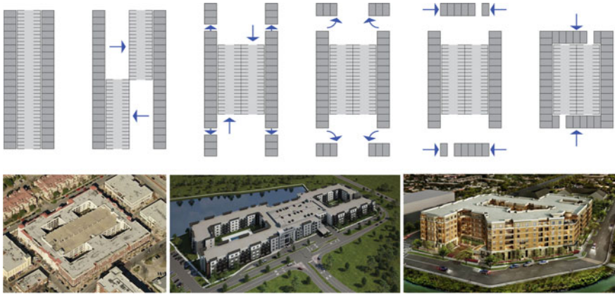
Fig. 11. Diagram of formation of Texas doughnut ( above ) (James 2017); images of typical Texas doughnut formations ( below ). Images from unknown authors, web references listed from left to right ([Texas Donut] [image] n.d)
