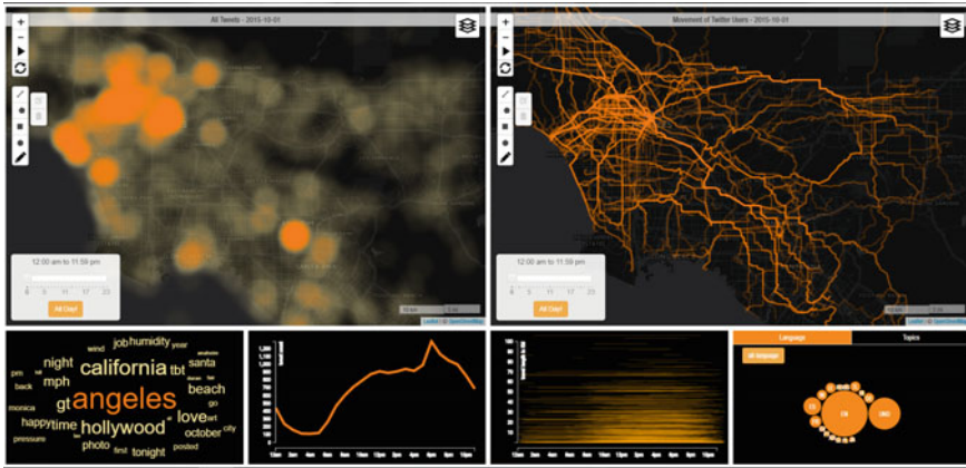
Fig. 3. Urban Activity Explorer, a visual analytic interface showing Los Angeles County. Heat map of tweets location ( top left ), flow map ( top right ), word cloud, timelines and language/topic views ( bottom )
