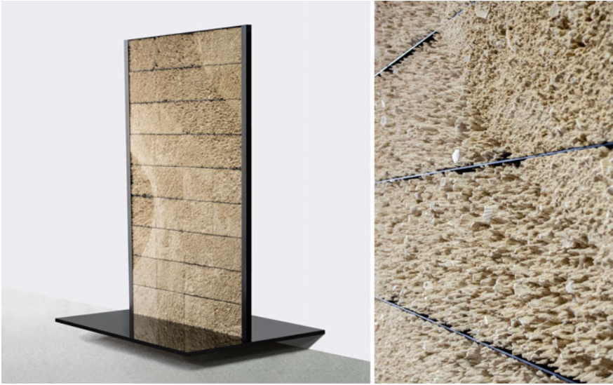
Fig. 7. The prototype wall is a 1.80 m \times 1.20 m structure comprised of 36 individual 25 mm thick limestone plates ( left ). Detail of wall ( right ). ©ICD, K. Rinderspacher
