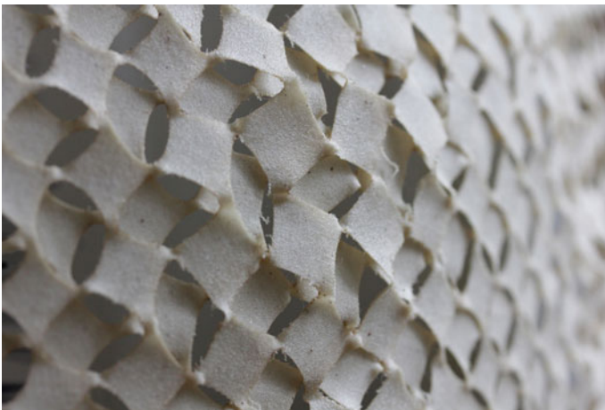
Fig. 19. Multi-layered auxetic structure made out of textile and epoxy resin forming a positive Gaussian curvature (maximum openings 22 mm)
