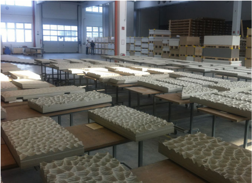
Fig. 7. Manufactured unique panels in the off-site workshop. Photo by Peuckert
