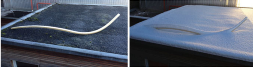
Fig. 17. Pictures of the tested acetylated double-curved wooden lath after fabrication ( left ) and exposed to temperature and hygrometry variation ( right )
