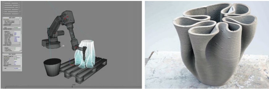
Fig. 13. Left processing of an outcome produced by proposed IDE by the manufacturer. Right prototype demonstrating the application of the proposed method. Printed at the RexLab, Institute of Experimental Architecture, at Innsbruck. Images courtesy Johannes Ladinig
