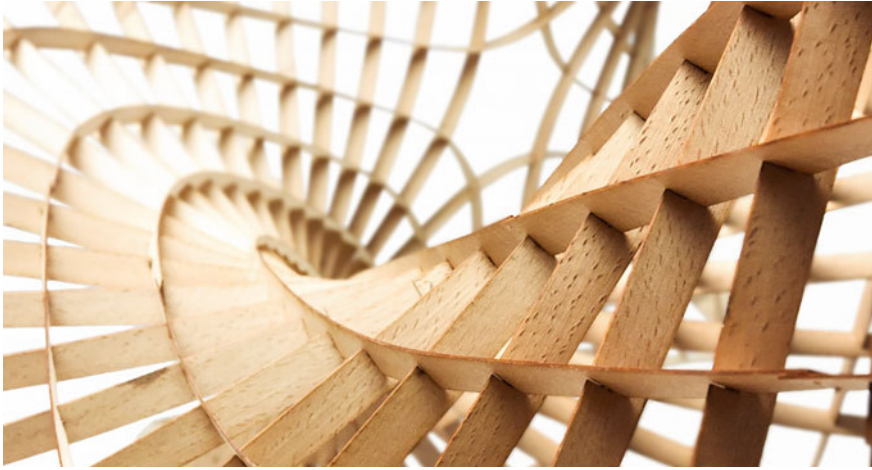
Fig. 1. Grid structure based on asymptotic curves: The model is built from straight strips of beech veneer. All joints are orthogonal. Image Denis Hitrec
