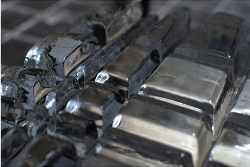
Fig. 7. Melting test #3—the ice formwork
