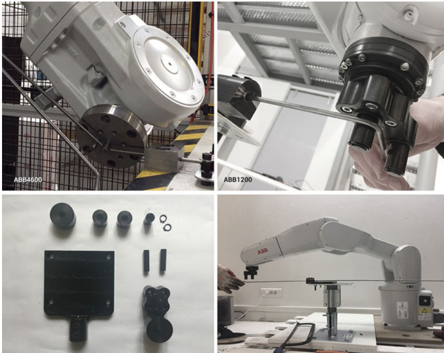
Fig. 8. From Left Top: Evolution of the toolhead and customization of equipment: Toolhead 1.0 for robotic arm ABB 4600; Toolhead 2.0 for the robotic arm ABB 1200 which is customized according to different bending radii, different rod size and its topology; Overview of the toolhead elements; stand-alone and single-support rod holding station
