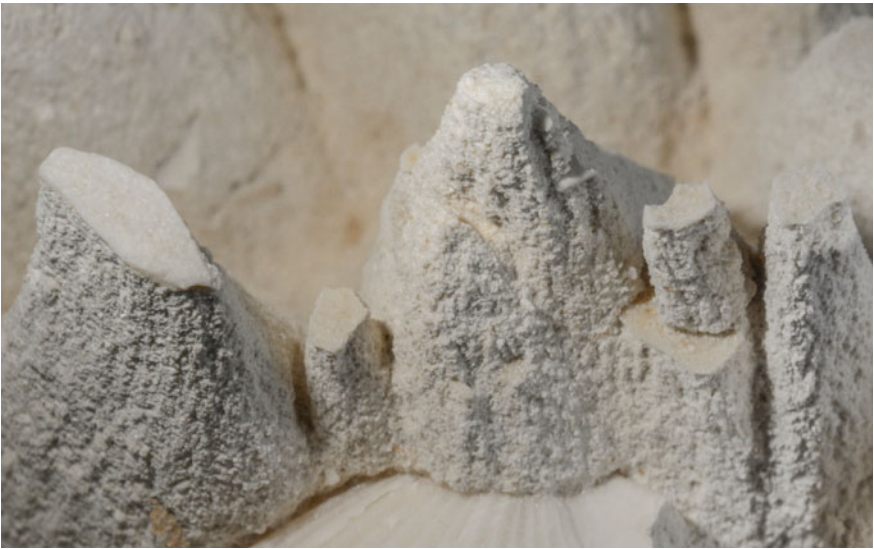
Fig. 2. Detail of erosion morphology as the calcium-based fragments impede the water. ©ICD, K. Rinderspacher
