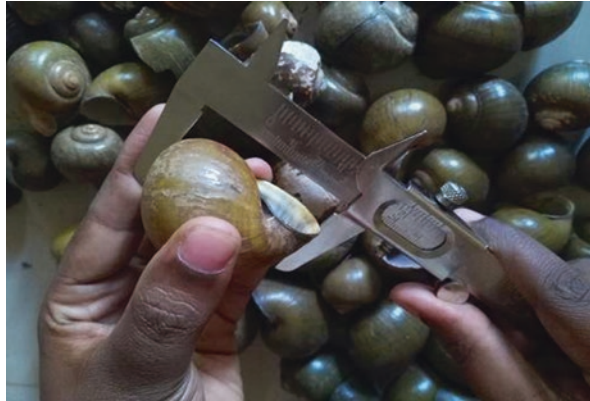
Fig. 7.8 Measuring shell size with vernier calipers
