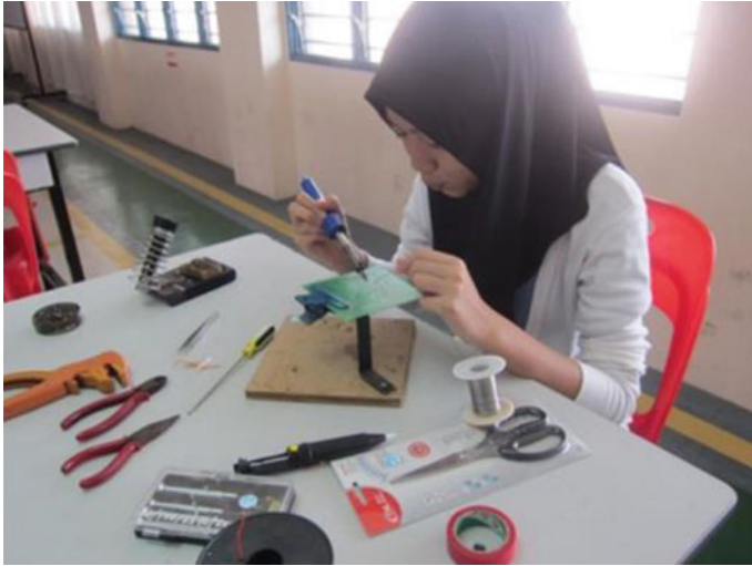
Fig. 4 Student soldering the preamplifier
