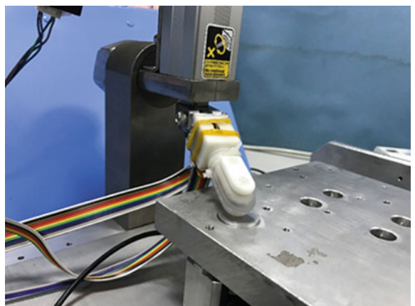
Fig. 11 Pressure calibration of finger sensor
