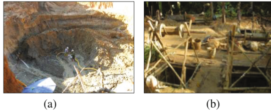
Fig. 2. Mining methods (a) Open pit mining method (Inn Bye), (b) Square pit mining method (Lebin Twin)
