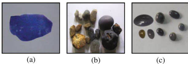
Fig. 2. (a) Sapphire crystal (rough), (b) Rough crystals of sapphire, (c) Cabochon cut sapphires
