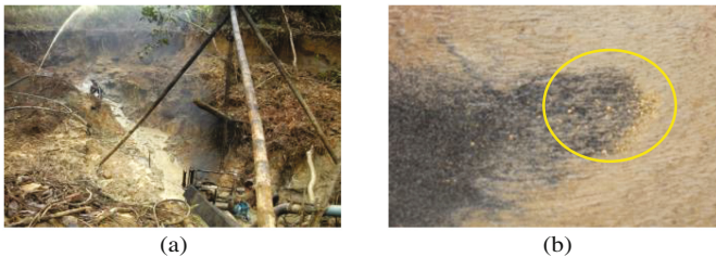
Fig. 6. Sample Worksite 5: (a) Recovery of byones by water sluicing method, (b) Gold particles
