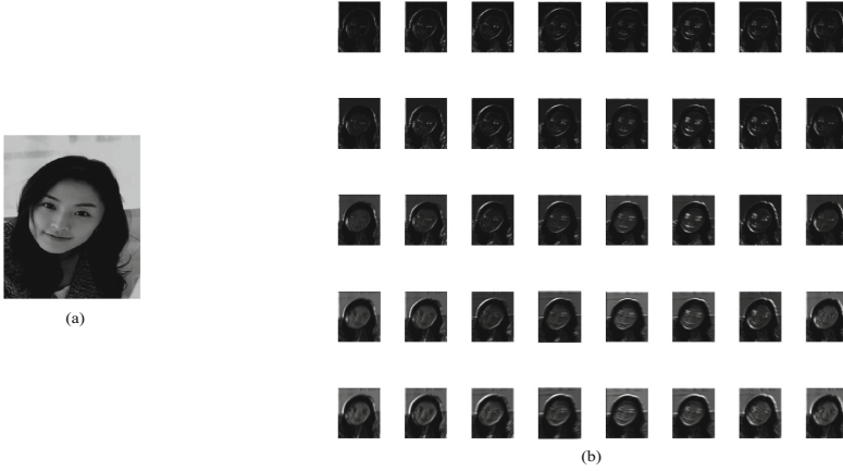
Fig. 2. (a) is the original image of the input. In (b), we show 40 filtered face images which include five scales and eight directions in different frequency bands extracted from the original image features.
