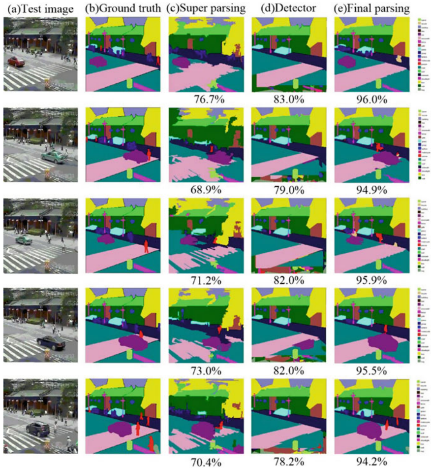
Fig. 4 The results of our approach in the video images. Column a is the test images; b is the ground truth; the superpixel parsing results are (c); d is the exemplar parsing results; and e is the final parsing results which combine (c) with (d)
