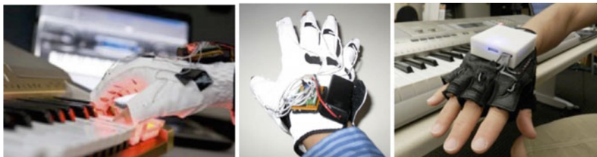
Fig. 6 Vibrating motors of Mobile Music Touch cue which fingers to play the piano
