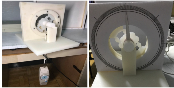
(a) installation of the revolute joint (b) testing of the revolute angel
