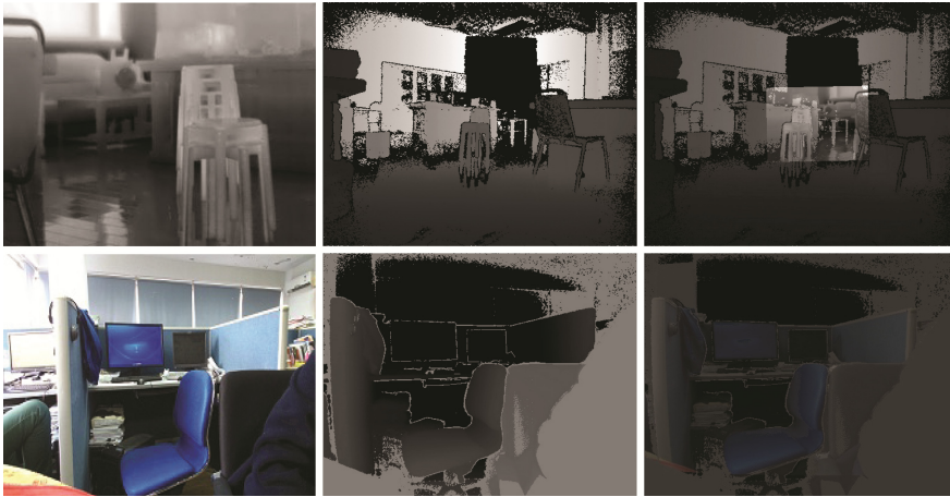
Fig. 2. The results of registration. First row: left column is original infrared images, middle column is original depth images, right column is registered images. Second row: left column is original color images, middle column is original depth images, right column is registered images.
