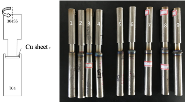
Fig. 4. Schematic diagram of FSW with middle layer of copper and actual picture of 304/TC4
