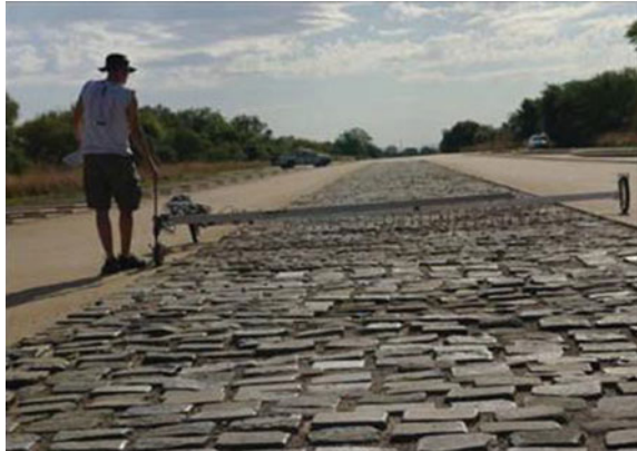
Fig. 4.4 Can-can profilometer measuring the Belgian paving (Becker and Els. 2014)
