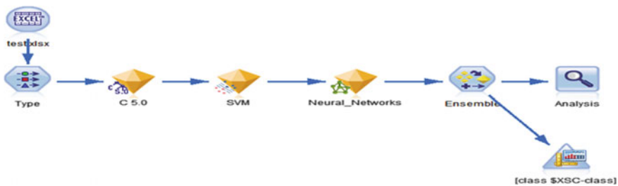
Fig. 7 Ensemble model for network intrusion detection system
