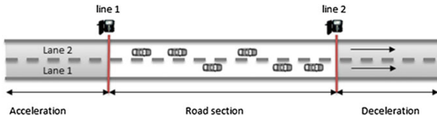
Fig. 1 Schematic representation of the observed road segment with marked lines for vehicle passage time readings
