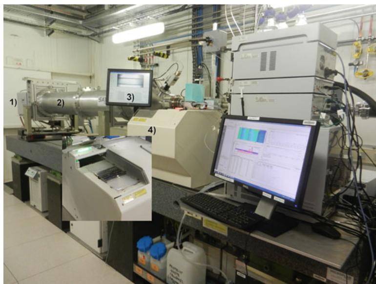
Fig. 4.1 Experimental setup at the ESRF BioSAXS beamline BM29. This experimental facility is dedicated to SAXS measurements of samples in solution offering both Static (batch) operation and online SEC measurements (both HPLC and FPLC). X-ray scattering images are acquired using a Pilatus 1 M detector 1 Air scattering is avoided by using an evacuated flight tube 2 A touch screen monitor 3 allows easy control of the dedicated sample changer 4 Inset photograph shows the sample changer from the top with sample storage opened
