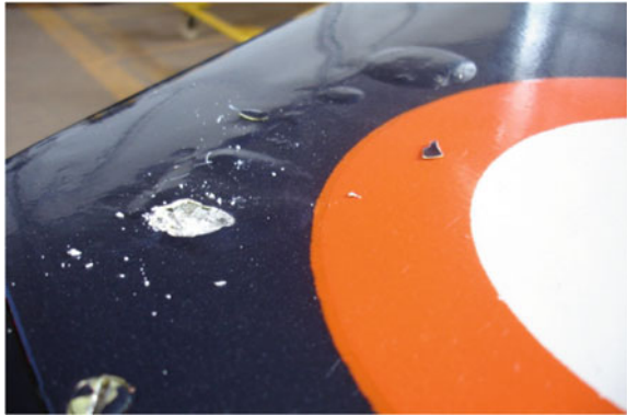
Fig. 10 Change in the wing profile due to local bulging
