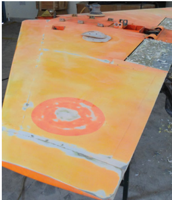
Fig. 11 Corrosion at wing and control surfaces
