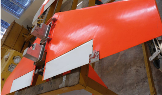
Fig. 12 Wing after repair and painting
