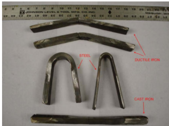
Fig. 2 Relative deformation in a 180° bending test [2]
