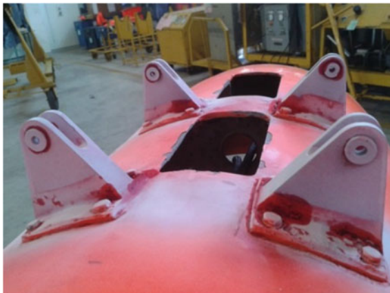
Fig. 6 Liquid penetration test of tail plane mounting brackets
