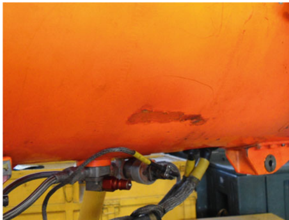
Fig. 13 Local indentation at fuel tank
