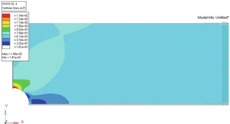
Fig. 3 von Mises stress contour of plate with single stress concentration zone
