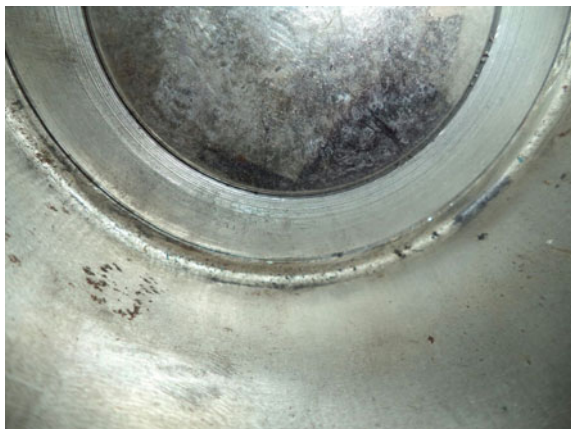
Fig. 4 Inner portion of the fixture to which the punch tool is clamped
