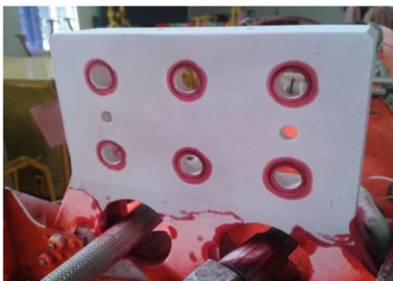
Fig. 7 Liquid penetration test of wing mounting bracket
