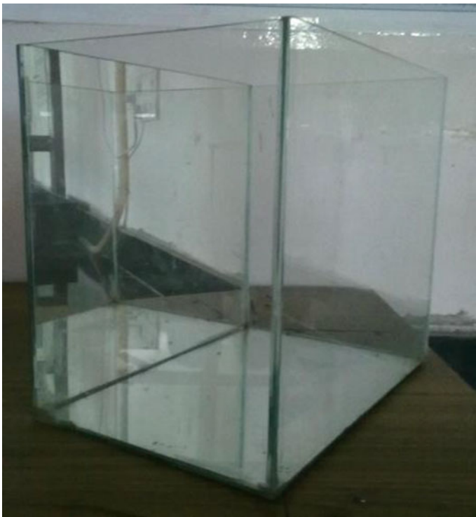
Fig. 5 Plexi glass cage with mirror
