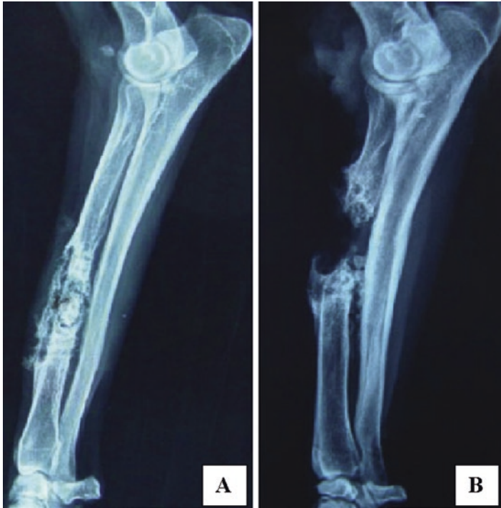
Fig. 4.15 Radiographic observation after 20 weeks in vivo: (A) CPC-fiber implant; (B) CPC control (Reprinted with permission from [91]. Copyright © 2012 Biomaterials Rights Managed by Elsevier)
