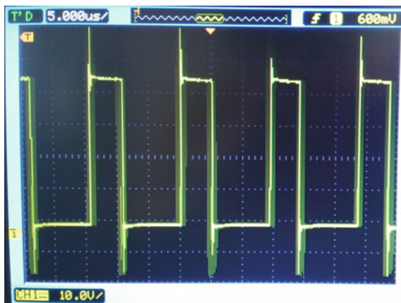
Fig. 6.8 Snapshot of the oscilloscope screen at 70 kHz MAS. The spinning signal is monitored after 1 ms trigger with the persistent mode. The jitter ( \pm 0.5 \mu\text{s} ) represents the spinning fluctuations of 250 ppm
