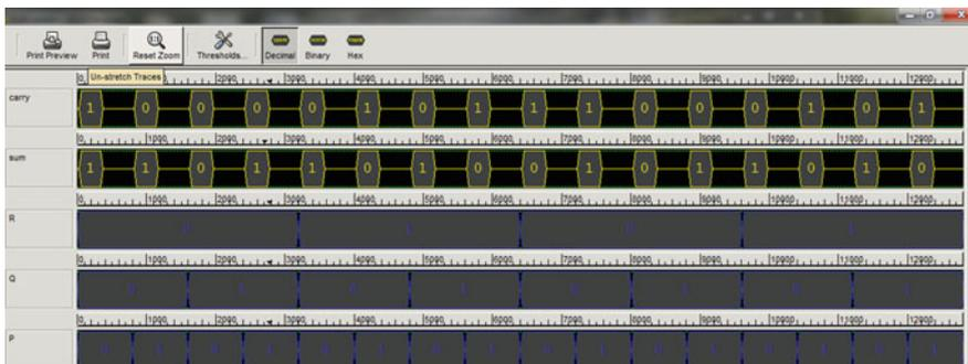
Fig. 15 Simulation of full adder using half adder
