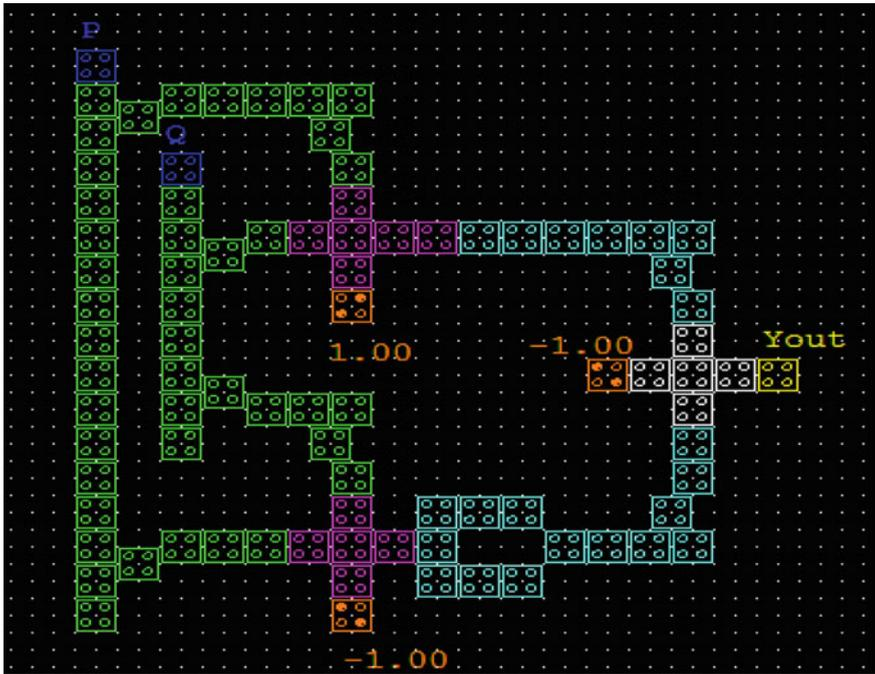
**Fig. 10** Layout of EX-OR gate
