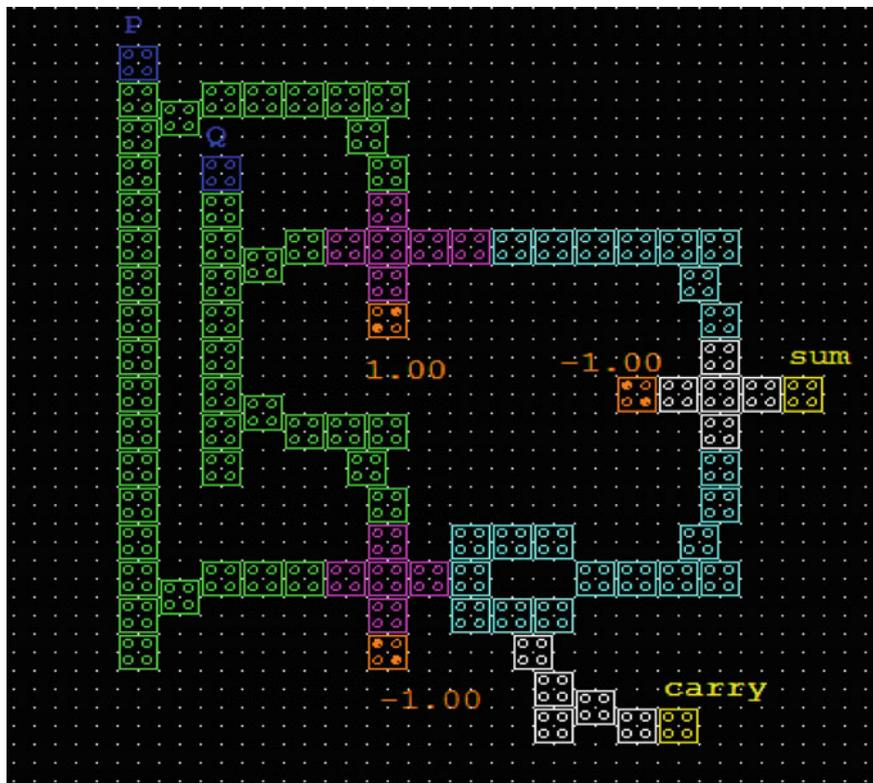
Fig. 12 Layout of half-adder using coplanar EX-OR gate
