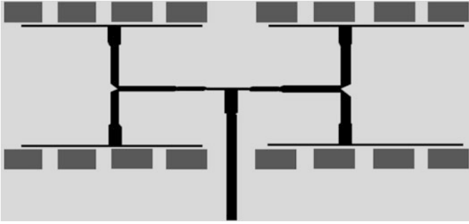
Fig. 2 Geometry of the proposed array ( 8 \times 1 )
