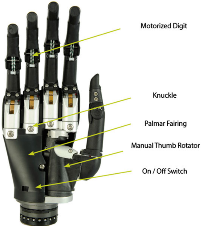
Fig. 7 Internal specification of prosthetic hand [8]
