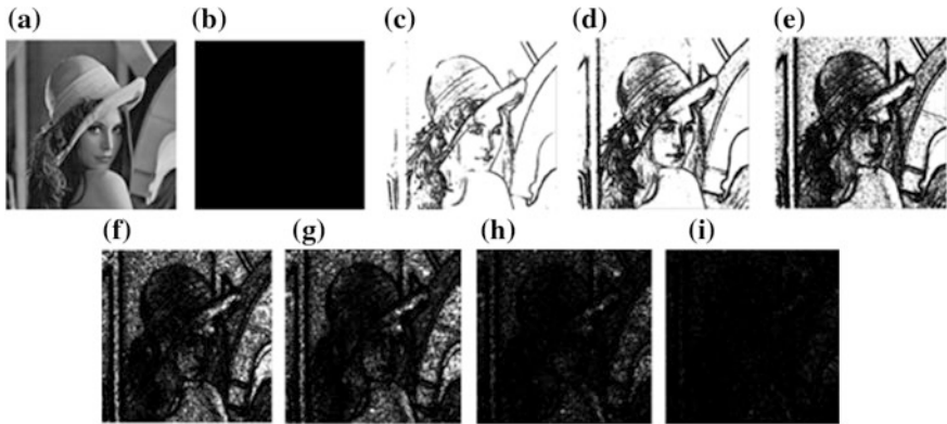
Fig. 2 a Original image, b threshold = 0.00, c T = 0.01, d T = 0.02, e T = 0.04, f T = 0.09, g T = 0.10, h T = 0.20, i T = 0.50
