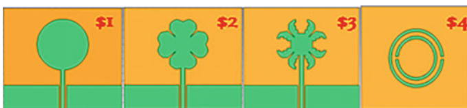
Fig. 1 Design evolution of the antenna proposed
