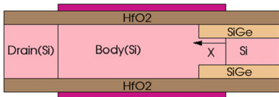
Fig. 1 Schematic view of DGTFET with extended SiGe/Si source structure. X is the encroachment of SiGe (p +) under the gate
