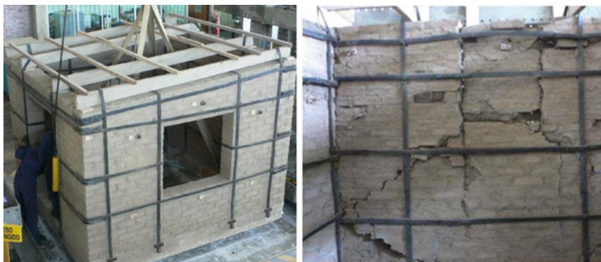
Fig. 12 Shaking table test on an adobe model strengthened with tire straps [58]
