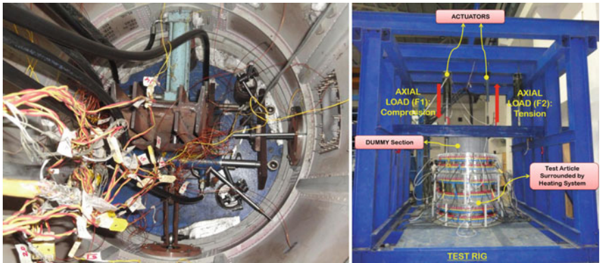
Fig. 9 Internal 90° loading arrangement and the complete test setup
