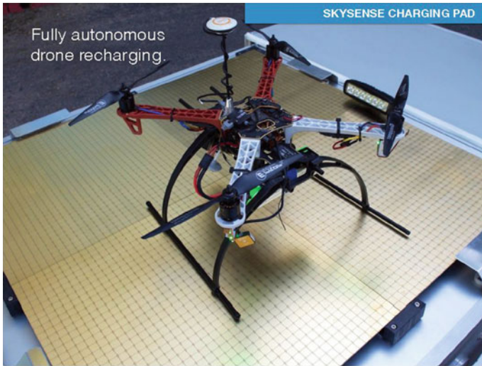
Fig. 2 Skysense company charging pad. (Source Skysense datasheet)
