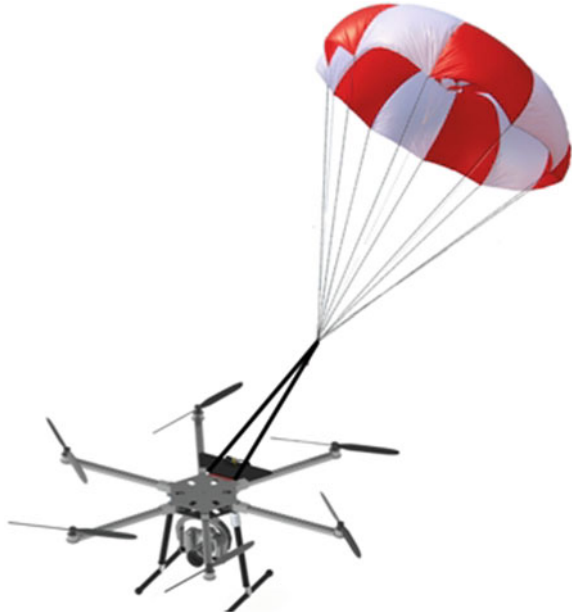
Fig. 8 Sample of parachute on a multicopter vehicle. (Source www.books.google.co.in )
