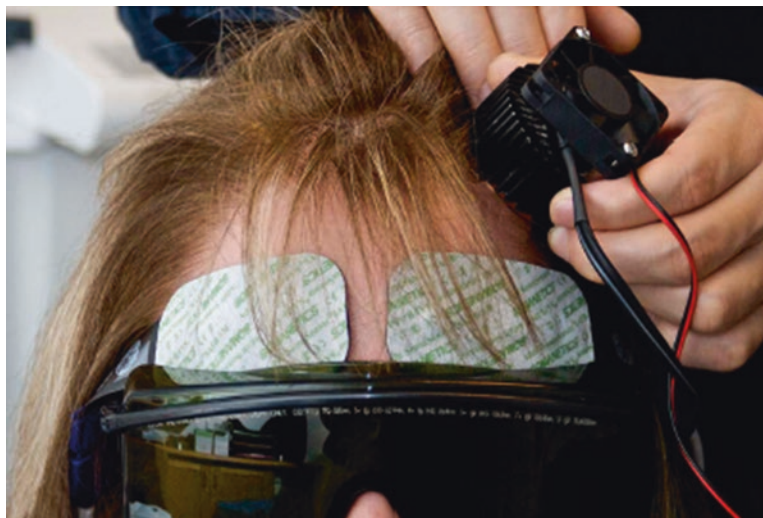
Fig. 18.5 Transcranial LED device. This device was used in the Schiffer et al. study for depression [45]
