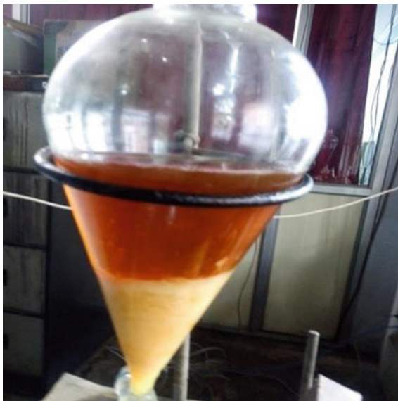
Fig. 2 Separation of oil and soap
