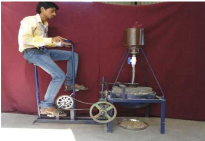
Fig. 4 Heap of end product at the outlet of pedal-operated flour mill
