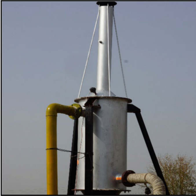
Fig. 3 Actual photographic view of shell and tube type heat exchanger
