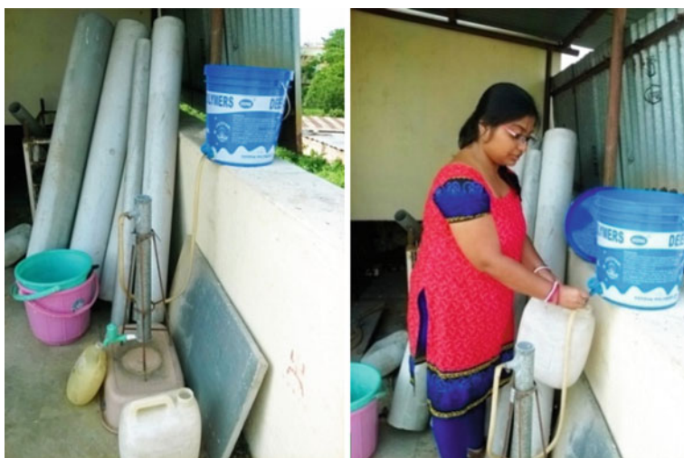
Fig. 15 Activated alumina filter set up
