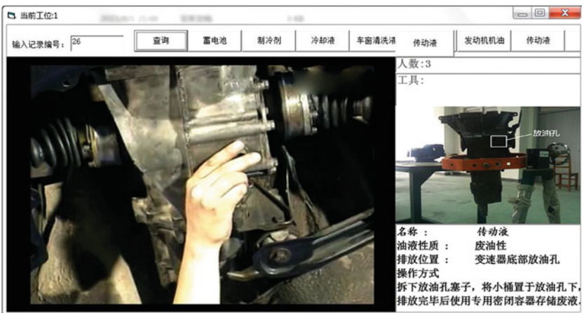
Fig. 7 Disassembly information output of the disassembly line station terminal
