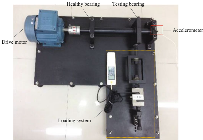
Fig. 4 Test rig for bearing
