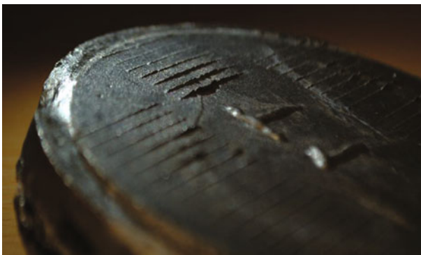
Fig. 5 Close up of the solidified aluminium at the bottom of disk 1 after the experiment was conducted. The melt enters the venting slot, but is released from the slot after the solidified casting is removed from the mould
