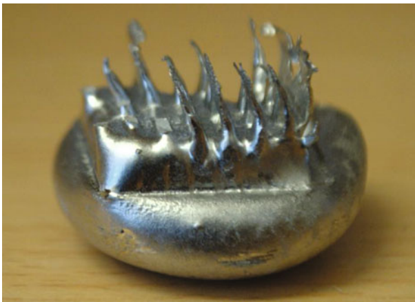
Fig. 6 A piece of aluminium which penetrated the 0.26 mm slot width group on disk 5 and solidified in the vacuum chamber
