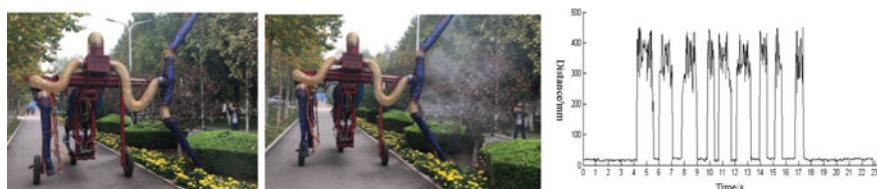
Fig. 4 Test chart of target spray and signal waveform
