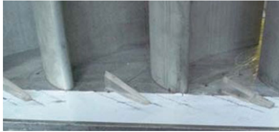
Fig. 7.22 Streamwise vortex generator mounted on the end wall [27]
