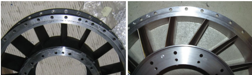
Fig. 8.15 EGV layout schemes: conventional scheme (left), leaning scheme (right) [76]
