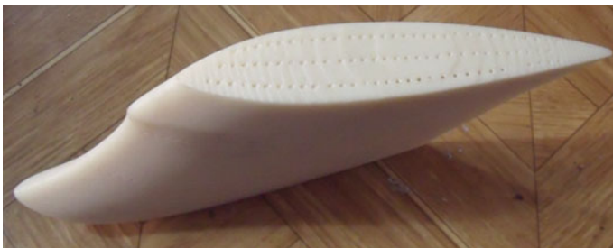
Fig. 6.114 Swept strut in a intermediate turbine duct
