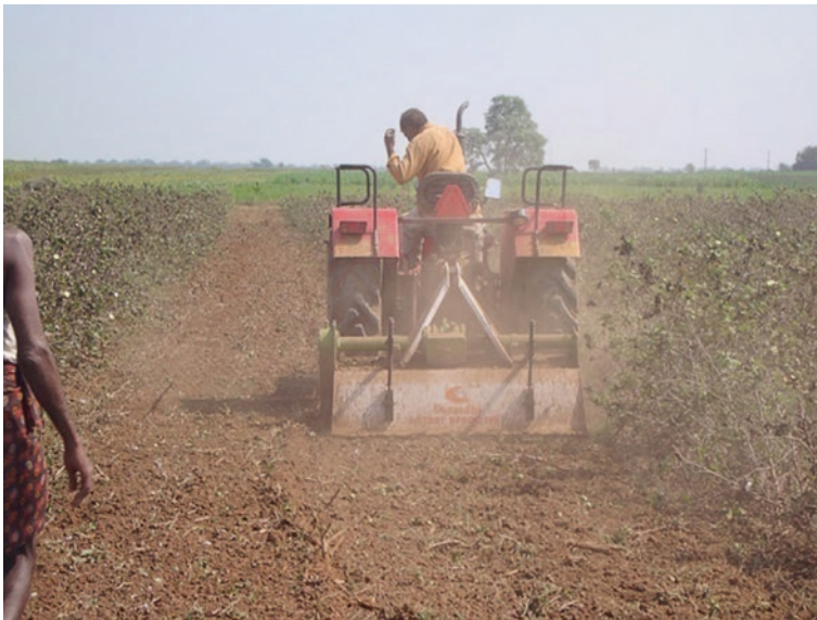
Fig. 6.6 Crop residue recycling into soil through rotavator
