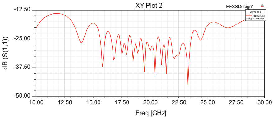
Fig. 7 Return loss of the bend with circular chamfrain corner at K -band frequencies
