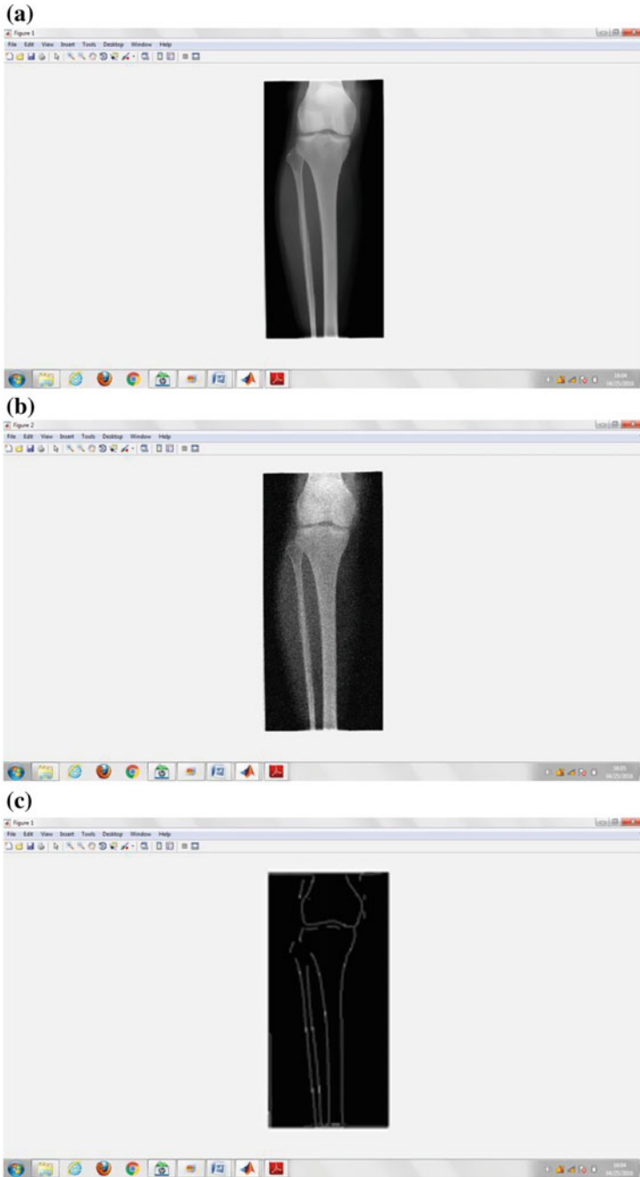
Fig. 5 a Original image, b image after undergoing Gaussian filter, c fracture detection using Sobel operator
