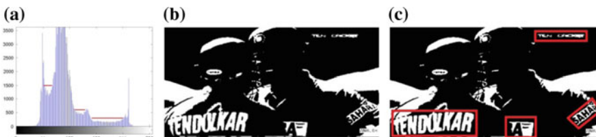
Fig. 3 Text area detection through conventional approach. a Histogram of input video frame. b Thresholding from one of the multiple threshold steps. c Detected text areas
