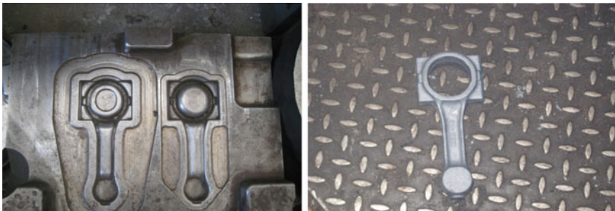
Fig. 5 Rectification of coining die and connecting rod
