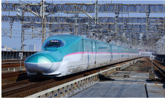
Fig. 5 Series E5 of East Japan Railways; Japan's highest speed operation at 320 km/h on 4000 m radius curve assisted by body inclination control realised together with E6, seen at the rear of the photo
