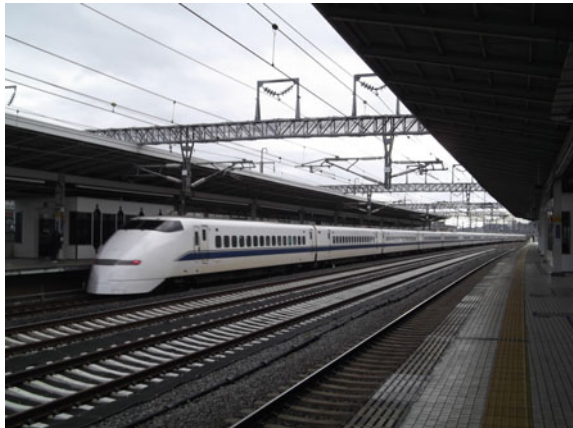
Fig. 1 Series 300 of Central Japan Railways; the world first high-speed trainset adopting regenerative braking
