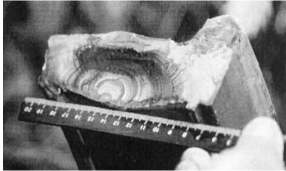
Fig. 7 Clear signs of the development of a fatigue crack in the fractured wheel rim, which caused the Eschede disaster of June 1998
