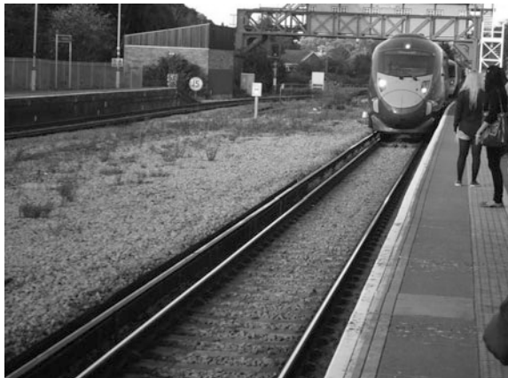
Fig. 5 Domestic services provided by the Hitachi Javelin trains: seen here operating on conventional track with a third rail 750 V DC current supply
