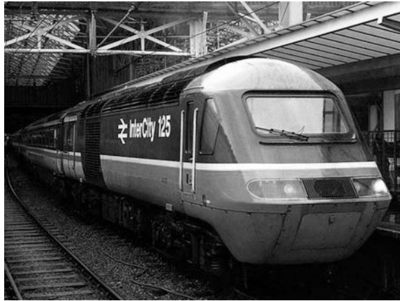
Fig. 3 The 125 high-speed train ( HST ): introduced in 1976 and still going strong today. It is the holder of the world's diesel traction speed record of 238 km/h
