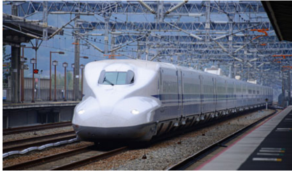
Fig. 2 Series N700 (14M2T) of Central Japan Railways; this can run at 270 km/h at 2500 m radius sharp curve by body inclination control. Figs. 2, 4 and 5 were provided by Mr. Chun-xiao LUO from Editorial Office of Railway Knowledge , China
