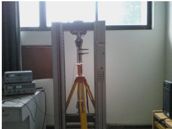
Fig. 6 Experimental setup for tension tests
