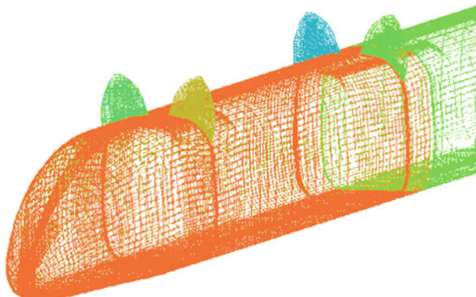
Fig. 4 Area meshes of the train and brake wings
