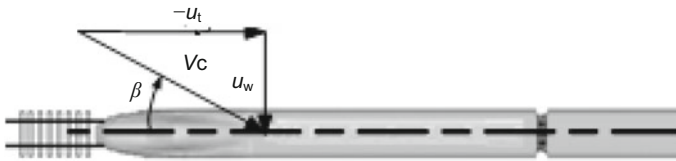
Fig. 4 Schematic diagram of the combined wind velocity. \beta : yaw angle; V_c : combined velocity
