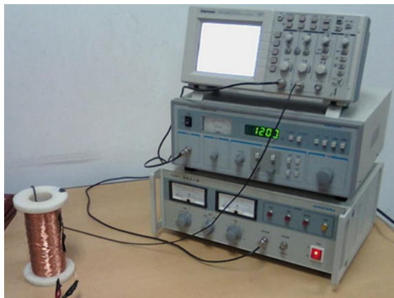
Fig. 3 Experimental setup for determining the relationship between V_{ME} (mV) and B (mT)
