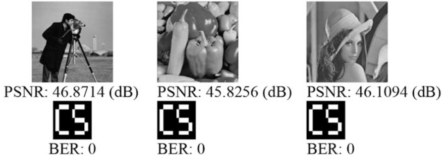
Fig. 4 Watermarked version images corresponding to Fig. 2 and extracted watermark against without attack case
