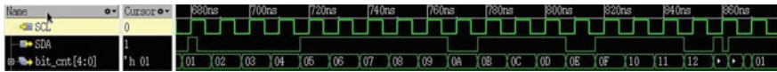
Fig. 9 Reading data from the slave using 10-bit addressing in Standard mode. (01) Start bit is set, (02–08) first part of slave address is mentioned, (09) ‘0’ mentioning write action, (0A) acknowledgment bit as ‘0’ i.e., slave is ready to accept data, (0B–12) 2nd byte address of the slave, (13) acknowledgment bit as ‘0’ i.e., slave is ready to send data to the master, (14–1B) data read from the slave, (1C) acknowledgment from slave to make repeated start
