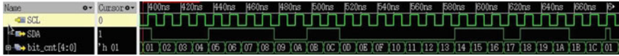
Fig. 8 Writing data into the slave using 10-bit addressing in Standard mode. (01) Start bit is set, (02–08) first part of slave address is mentioned, (09) ‘0’ mentioning write action, (0A) acknowledgment bit as ‘0’ i.e., slave is ready to accept data, (0B–12) 2nd byte address of the slave, (13) acknowledgment bit as ‘0’ i.e., slave is ready to accept data, (14–1B) data written to slave, (1C) acknowledgment from slave to make repeated start i.e., performing read action from the slave
