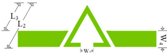
Fig. 1 Structure of open-loop triangular ring resonator coupled in series with transmission line
