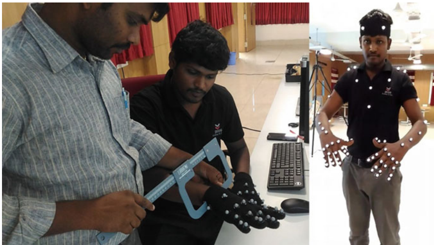
Fig. 4 Marker placement design and actual markers used for capturing the sign language
