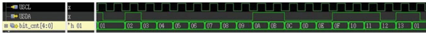
Fig. 10 Writing data into the slave using 7-bit addressing in UFM mode. (01) Start bit is set, (02–08) slave address is mentioned, (09) ‘0’ mentioning write action, (0A) acknowledgment bit as ‘1’ (ack signal is not required in UFM mode but to retain protocol bit pattern the ack bit is mentioned), (0B–12) data written to slave, (13) acknowledgment from slave which is always set as high
