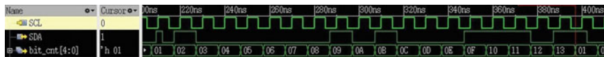
Fig. 7 Reading data from the slave using 7-bit addressing in standard mode. (01) Start bit is set, (02–08) slave address is mentioned, (09) ‘1’ mentioning read action, (0A) acknowledgment bit as ‘0’ i.e., slave is ready to accept data, (0A–11) data read from slave, (12) acknowledgment from slave to make repeated start
