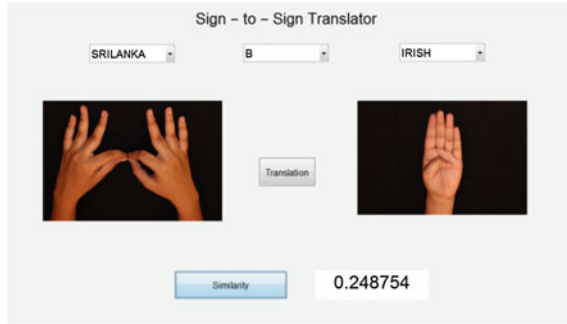
Fig. 7 Sign-to-sign translator between Sri Lanka and Ireland for sign B
