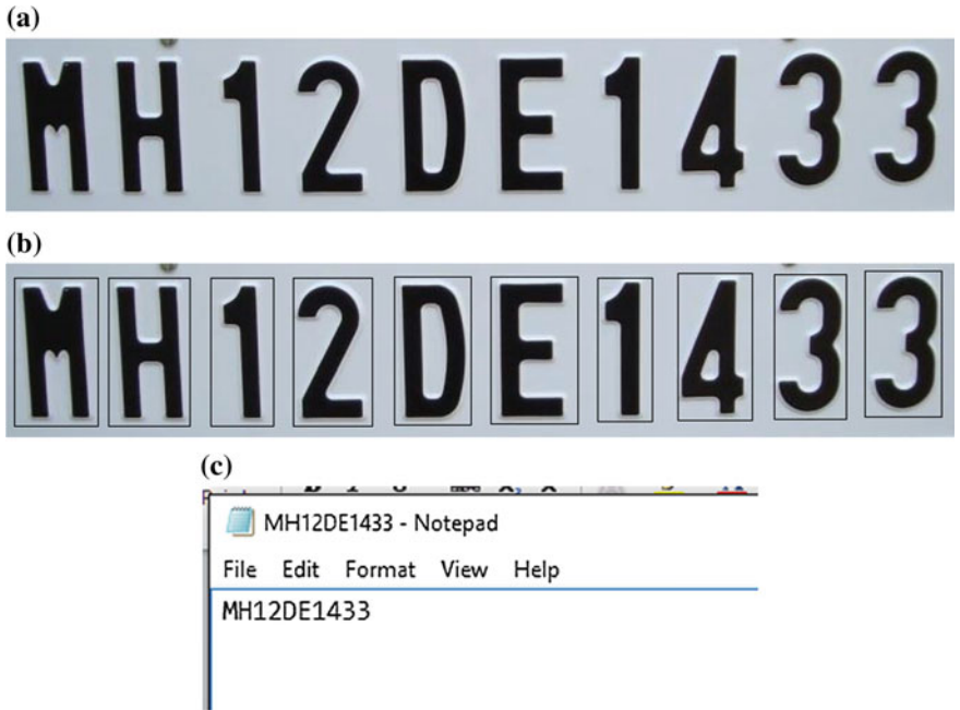
Fig. 6 a Sample input image; b Character extracted as blocks; c Output text file
