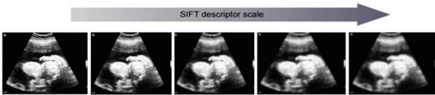
Fig. 2 Scale space of one image from training set. With increasing scale, it is observed that resolution of image decreases
