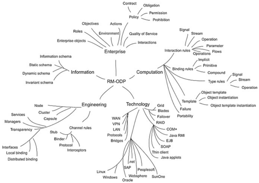
Fig. 11 Scale of complexity of the architecture viewing the communication dependency of RM-ODP [43] Source [4]
