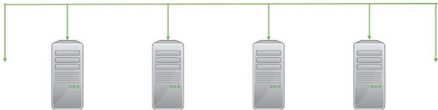
Fig. 5.2 Bus (or line) topology
