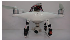
Fig. 5. DJI Phantom 4 armed with gas sensors.
