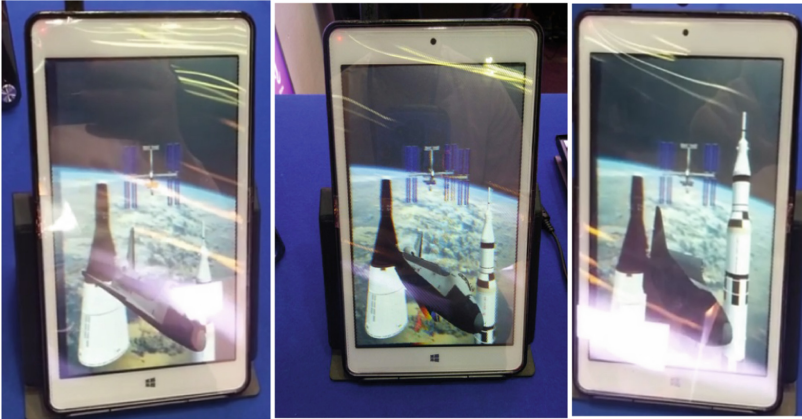
Fig. 7. Showing the 3D object displayed through the lenslet case from different viewpoints. Though not recognizable due to the 2D paper format the content appears in 3D in real environment.
