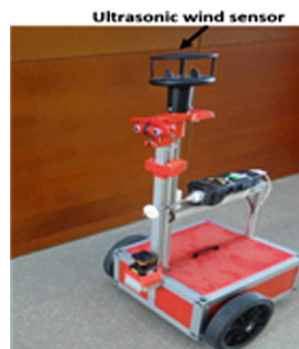
Fig. 3. Ultrasonic wind sensor mounted on wheeled base gas tracking robot [6]
