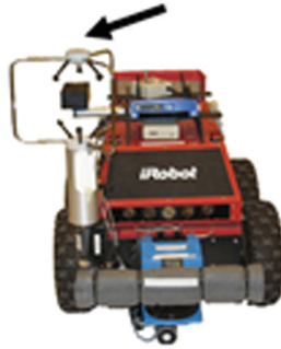
Fig. 4. Three-axis ultrasonic wind sensor mounted on wheeled base gas tracking robot [6]
