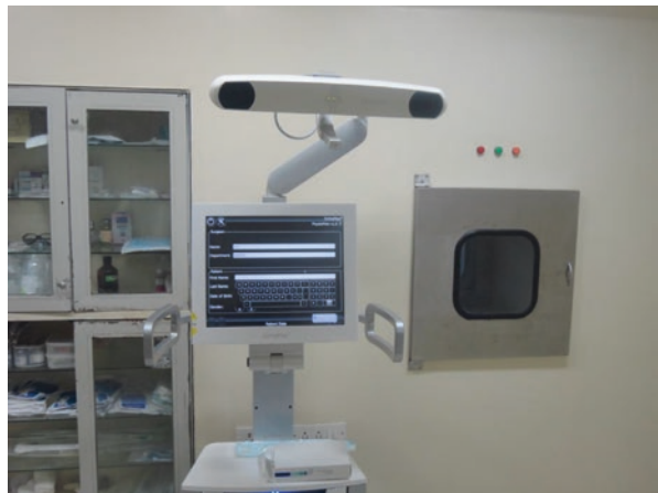
Fig. 9.2 Camera is adjusted in the right direction and distance from the operative site so it focuses on the sensors and data is shown on the screen
