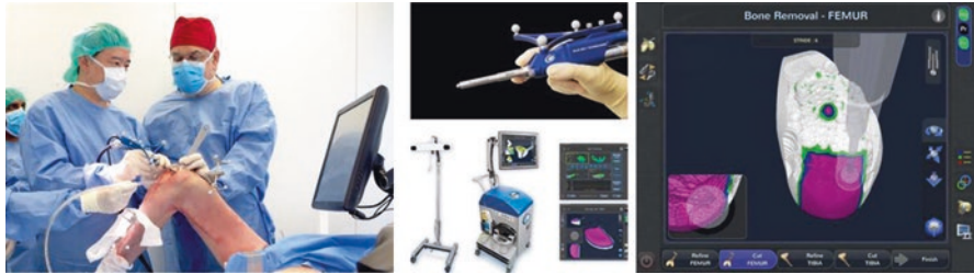
Fig. 6.2 The Navio Precision Free-Hand Sculptor (PFS) system
