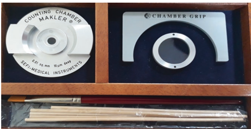
Fig. 5.1 Above photograph depicts the Makler counting chamber and cover glass with grid. This is a simple-to-use device for rapid and accurate sperm count and motility evaluation
