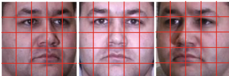
Fig. 2 Facial images are divided into local regions. Features are extracted based on each patch, thus the patch-based feature is invariant to pose
