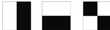
Fig. 7 Haar-like features used in branch networks. (©[2017] IEEE. Reprinted, with permission, from Ref. [25])
