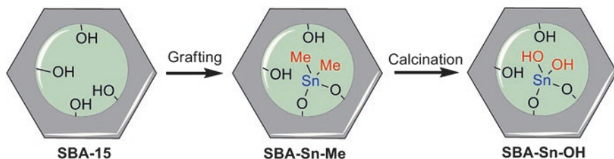
Fig. 1.11 Schematic route for synthesis of Lewis-Brønsted bifunctional SBA-Sn-OH (Adapted with permission from Ref. [77], Copyright © 2014 Royal Society of Chemistry)
