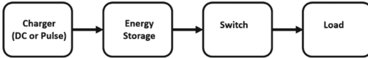
Fig. 15.1 The block diagram of a pulsed power system. The charger can be a DC voltage source or a pulsed source. The energy storage can be a capacitor, an inductor, or the combination of both. A switch allows the stored energy to transfer to a load, which, in bioelectrics applications, can be cell medium or a bulk of tissue
