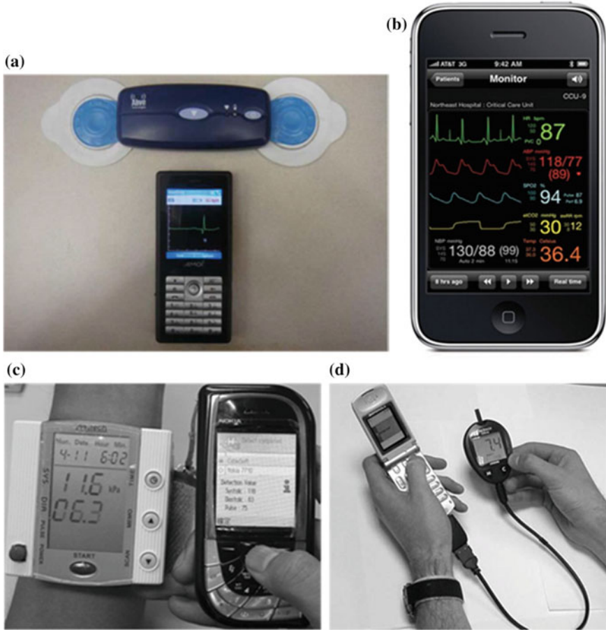
Fig. 4.3 Healthcare applications using Smartphones to monitor a ECG, b blood pressure, heart rate, SPO2 and body temperature, c blood pressure and pulse, d blood sugar level
