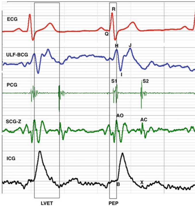
Fig. 2 Simultaneous recording of cardiac mechanical signals (middle three traces) and ECG and impedance cardiogram (ICG) signals as reference from a 36 years old male normal subject. The systolic time intervals of pre-ejection period (PEP) and left ventricular ejection time (LVET) are also shown. BCG was recorded from an ultra-low frequency bed and SCG was recorded in dorso-ventral direction
