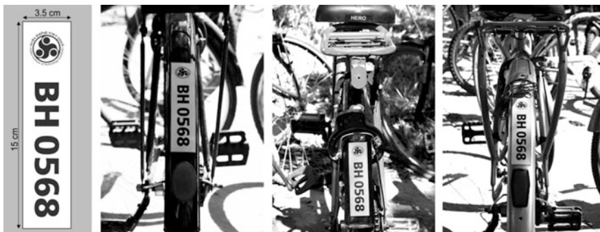
Fig. 4 Final proposed design and its placement on bicycle
