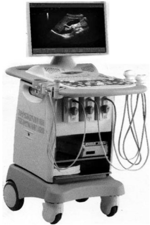
Fig. 1.10 Ultrasound equipment with multiple probes
